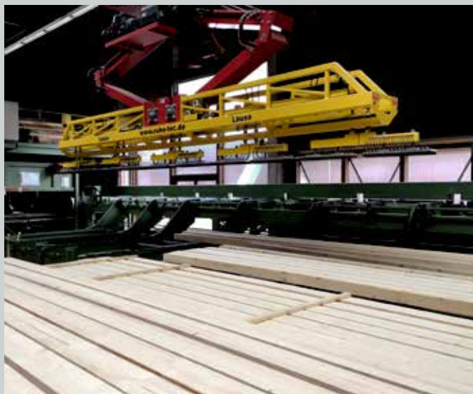
Schwenkbare Saugplatten Swivelling vacuum plates
