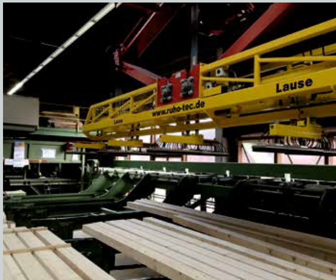
Schwenkbare Saugplatten Swivelling vacuum plates
