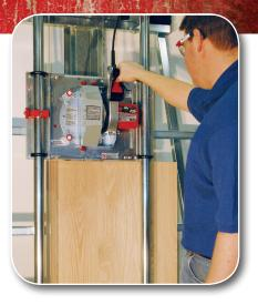
The C4 and C5 models are designed for customers who have limited floor space or require transporting the saw to the work site. Both models pack the same features as the full-sized models into a portable 5' frame. The C4 is ideal for cutting 4' x 8' sheets while the C5 can cut sheets 64" wide making rips and cross cuts safe and simple.
