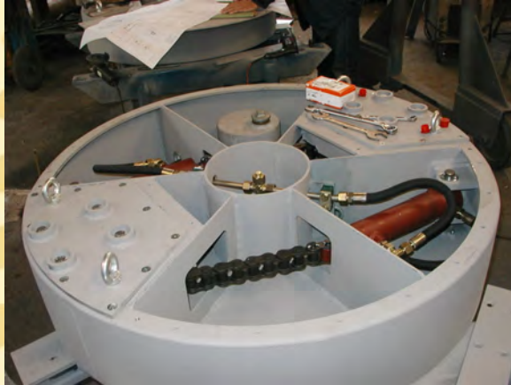
Rotor house during mounting of the hydraulic systems of rotor arms
