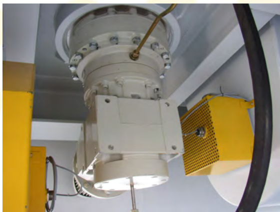
Planetary gear motor with integral hydraulic oil passage. Up to 200,000 Nm torque can be installed.
