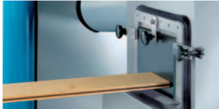
The VACUMAT® coating chamber makes all-over coating possible in one working process. Even undercut profile segments are coated with high application reliability.
