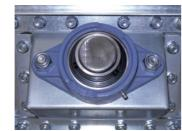
3 Low maintenance costs due to easily accessible lubrication points e.g. of the external bearings. Located safely and protected, they cannot be polluted, which extends their durability. Furthermore, all Schuko spare parts are available long-term and quickly.
