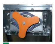
3 Operational safety. Improvement of failure safety by monitoring the transport chain and rotary valve with an inductive transmitter. (Optional)
