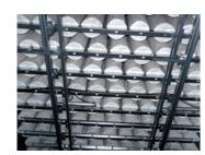
2 Increased filter surface allows malfunction-free performance of the extraction system. Raising the filter surface by 21% per element enables an even more effective strain of the filter material and prolongs the lifetime of the filter hoses drastically.
