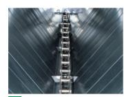
4 Reliable extraction achieved by high-quality chainextraction: reinforced design, no material build-up, self-tightening and maintenance-free. Wearresistant through steeper funnel
