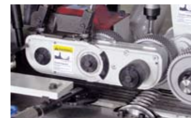
Pneumatic element for left spindle. Reduced distance between feed rollers.
