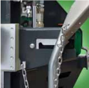
Ratchet of the lifter (Patent SI 23537)
