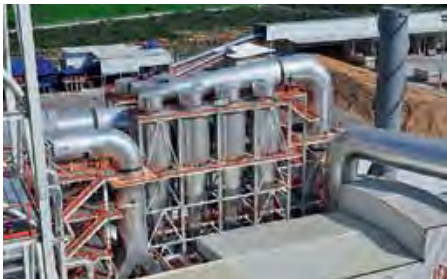
Cyclones of a 76 MW energy plant
