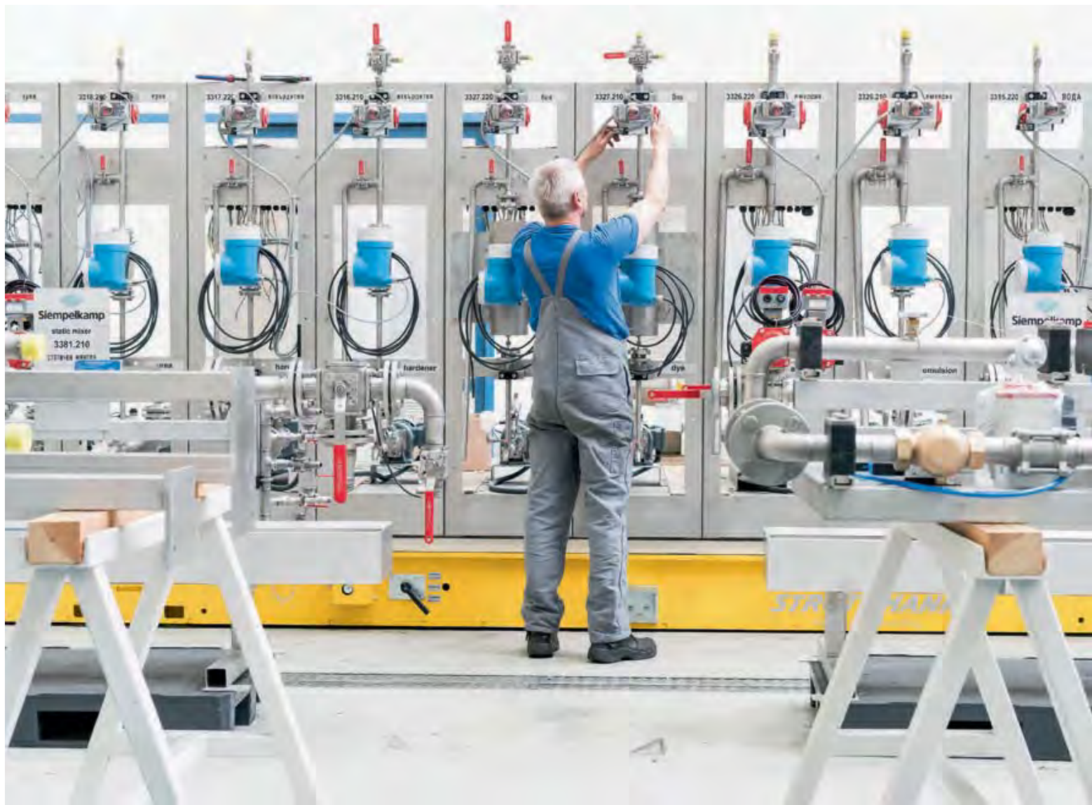
Assembly of the modular designed chemical metering system
