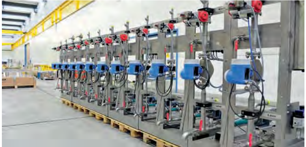
Assembly of the modular designed chemical metering system
