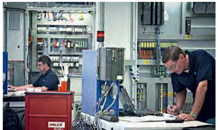
ATR specialists carrying out the final checks of switch cabinets
