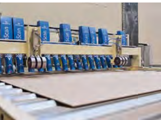
SicoScan ultrasonic measurement system for blister and delamination detection with thickness gauge
