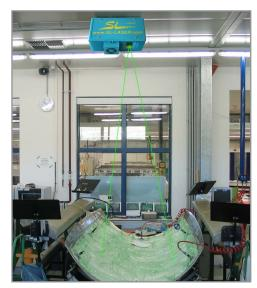
SL-Laser Systems makes time-consuming and inaccurate hand measuring and templating a thing of the past. Gone are the bulky manual templates and cumbersome mylars, replaced with a laser-crisp pattern of bright green light.
