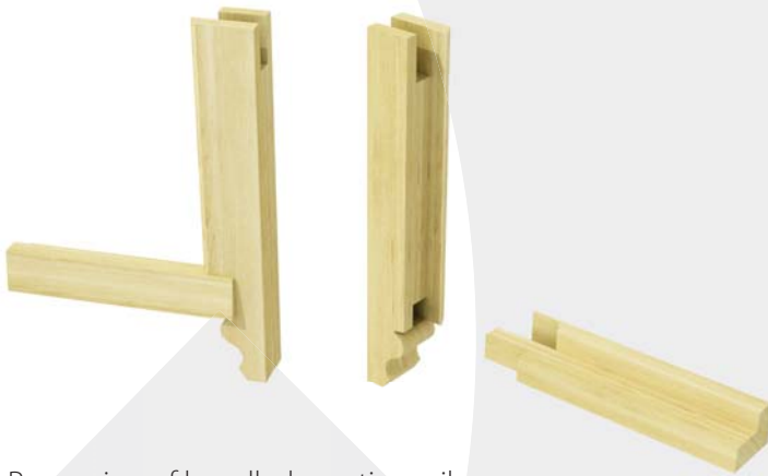
Processing of bevelled meeting rails and stiles with horn details
