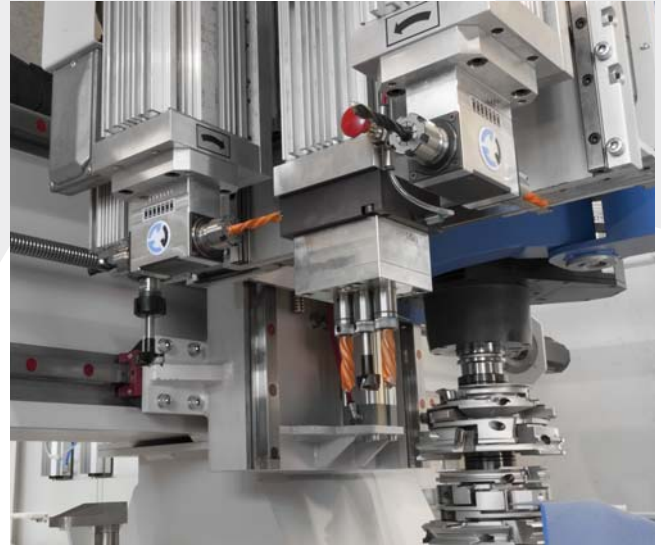
Tenoning spindle with drilling units
