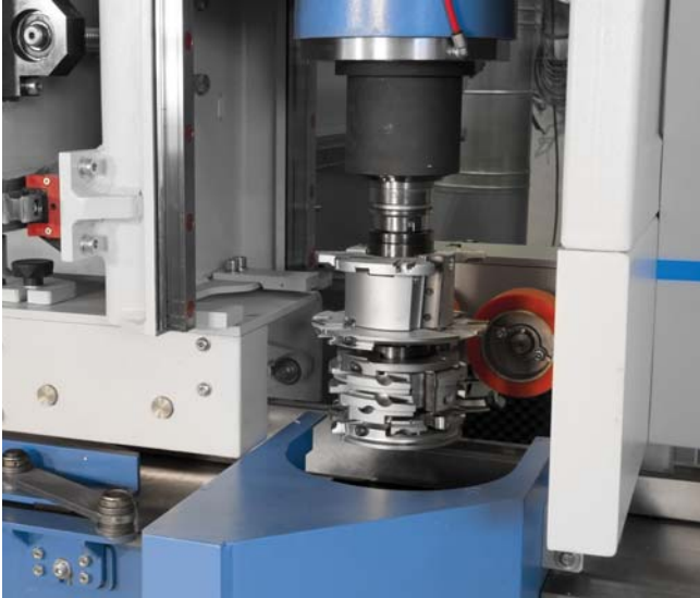
Profiling unit working from both sides
