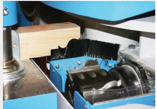
Horizontal milling unit for horns and trenching operations
