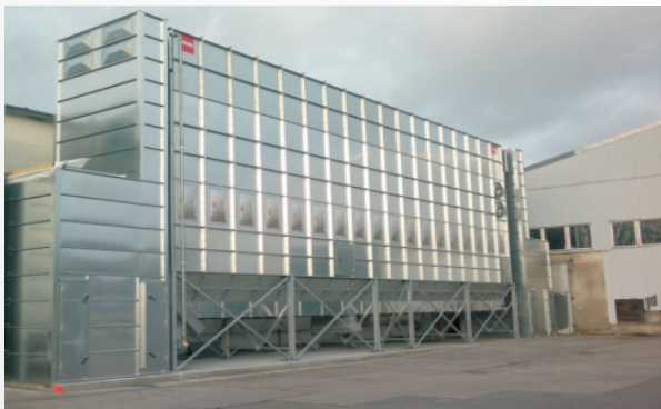
Line filter with reverse-air cleaning
