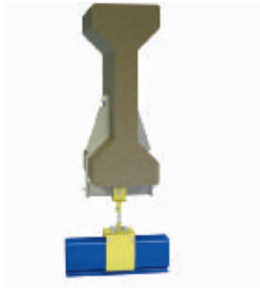
2. Example of a suspension for curved concrete beams. The bracket supports the steel tube to which a U-suspension is attached.
