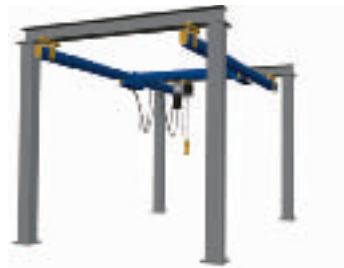
LR120/170 steel profile system in a low built system. SWL up to 1500 kg with reinforced profiles. The freestanding, portal suspending construction is an alternative to ceiling and wall suspension.
