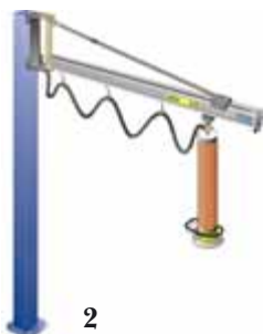
2. Jib arm, mounted on column. Max capacity 125 kg. Radius of action 240 degrees. Arm bracket measures 575/860 mm. Standard column height 3610/3840 mm.
