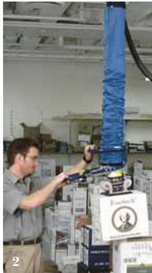
2. Retailers of alcoholic beverages use the VacuEasylift to handle boxes, crates and kegs. These units are equipped with a specially designed handle and are delivered with lightweight, lowbuilt aluminium jib cranes and crane systems.
