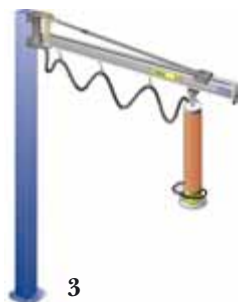
3. Low built jib arm, mounted on column. Max capacity 40 kg. Radius of action 240 degrees. Arm bracket measures 300 mm. Standard column height 3000 mm. Also available as wall mounted jib cranes.
