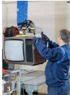
3. Recycling of TV sets and other electronic devices. A rapidly growing area of application with VacuEasylift.
