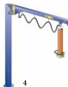
4. Inverted jib arm, mounted on column. For extremely low headroom. Max capacity 80 kg. Standard column height 3130 mm. Arm profile in steel. Also available as wall mounted jib cranes.
