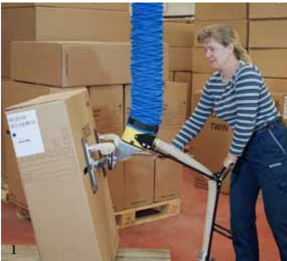
1–2. An angle adapter with handle solves the problem of picking up a vertically positioned object and moving it into a horizontal position.
