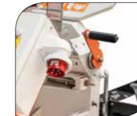
Sawyer has quick and easy access to: head up and down crank, blade guide arm, and blade control lever.
