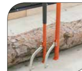
Cant Hook (option) is a traditional tool to roll, lift, move, and pivot logs. Available lengths of handle: • 70 cm • 120 cm
