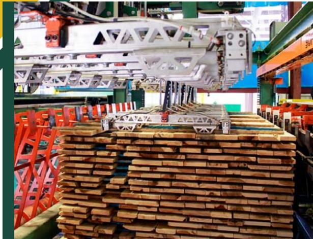
The TS Accu-Placer was designed with modularity in mind. Systems are customizable for placement rates of 150+ sticks per minute. Combined with 12+ layers per minute of placing capacity, the TS Accu-Placer becomes one of the fastest, most accurate stick placers on the market today.
