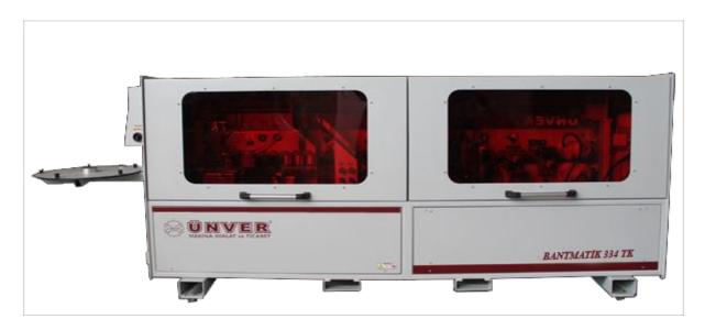
MACHINE LENGTH 3,3 METERS. IT HAS 4 UNITS. WORKING SPEED 15 METER/MINUTE.
