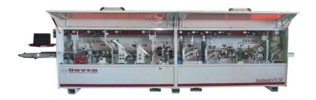
MACHINE LENGTH 4,7 METERS. IT HAS 6 UNITS. WORKING SPEED 9 - 18 METER/MINUTE. (WHEN TRIM UNIT WORKING 9 M/MIN). YOU CAN CONTROL ALL UNITS WITH COMPUTER EASILY. YOU CAN SEE MALFUNCTION, NUMBER OF PIECES, PVC BAND METERS AND MAINTENANCE WARNINGS.
