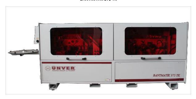
MACHINE LENGTH 3,7 METERS. IT HAS 5 UNITS. WORKING SPEED 15 METER/MINUTE.
