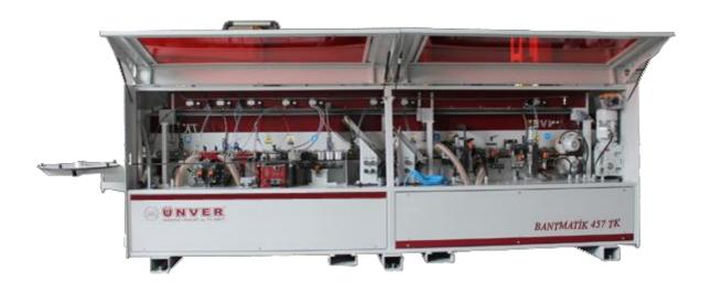
MACHINE LENGTH 4,5 METERS. IT HAS 7 UNITS. WORKING SPEED 15 METER/MINUTE.
