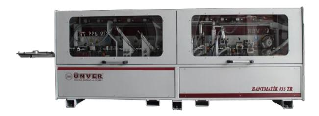
MACHINE LENGTH 4,3 METERS. IT HAS 5 UNITS. WORKING SPEED 12 METER/MINUTE.
