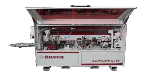
MACHINE LENGTH 2,4 METERS. IT HAS 3 UNITS. WORKING SPEED 15 METER/MINUTE.
