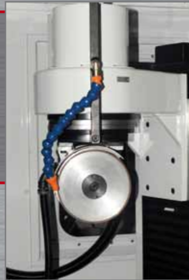
Motorized work head for O.D. grinding or circular saw sharpening.
