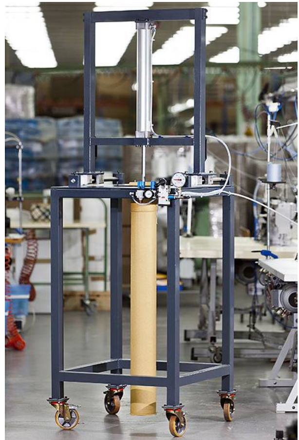
Fitting for hole plate assembly test.
