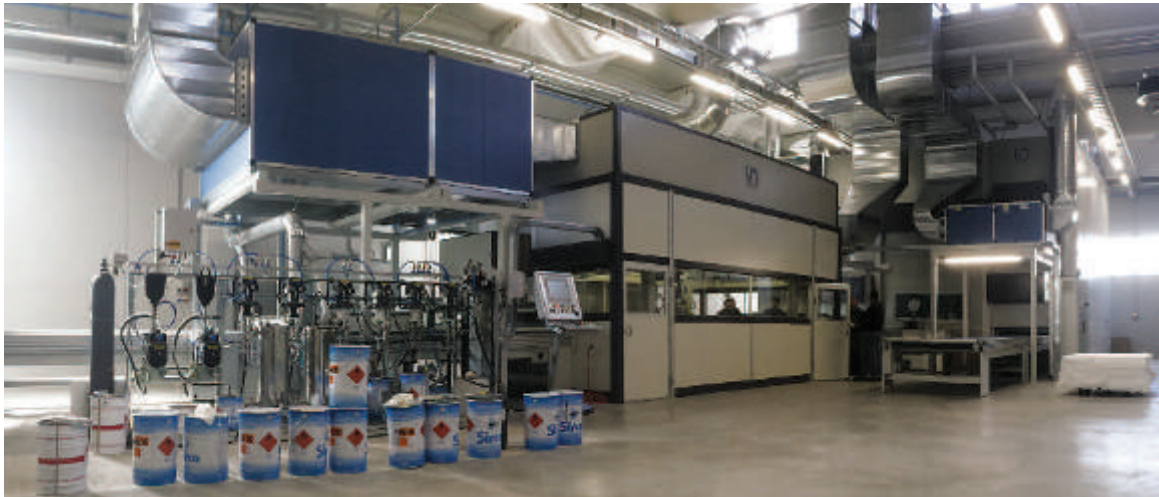
↑ Robot finishing line with Cobra 2 and vertical oven.
