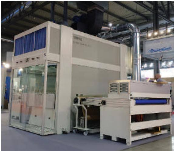
↑ Robot finishing line with Cobra 2 and vertical oven.
