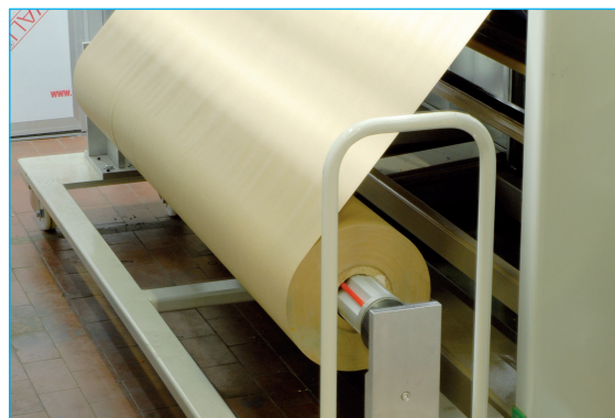
Dettaglio bobina in carta - Coil-uncoil paper system
