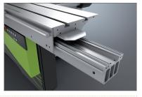
The cross cut fence with telescopic device is designed for cuts up to 3,200 mm and 90° guarantee.
