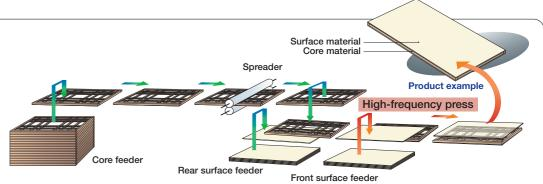
The core material automatically fed from the core feeder is transferred from the spreader feeder conveyor to the spreader and then coated with adhesive. The rear and front surface materials, which have been automatically set in the high-frequency panel joining machine, are then automatically transferred with the conveyor belt to enable one worker to perform all operations.
