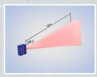
Laser projectors are able to project over longer distances with high precision using a Teleoptic.
