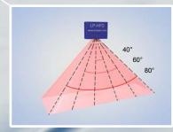
The projectors can be specified with fan angles up to 80°.
