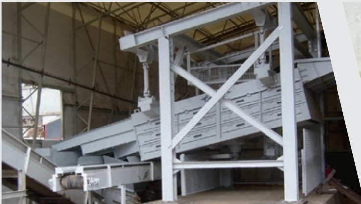
Oscillating screen for grain size classification of treated wood
