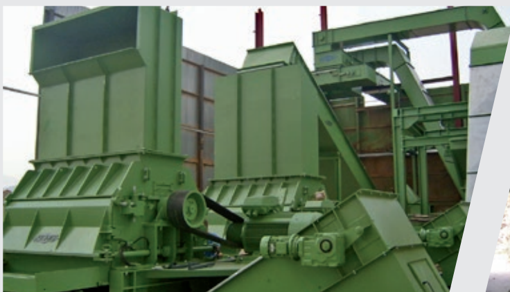
ZENO post-shredder type ZHM, in- and outfeed via chain conveyor
