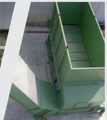
Chain dosing bunker with TKF chain conveyor
