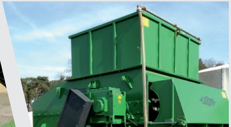
ZTLL for waste wood post-shredding with water injection
