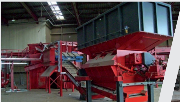
Pre-and post-shredding with metal separation
