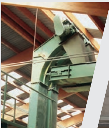
Chain conveyor for chips and sawdust
