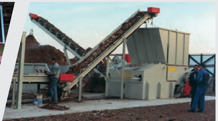
Pre-shredding with a single shaft shredder
