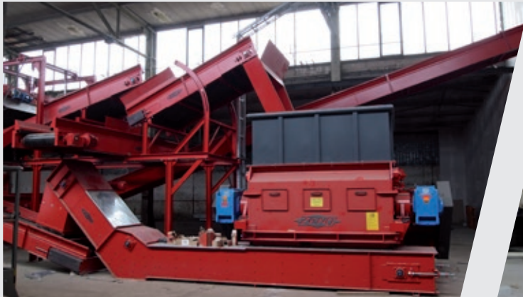
ZTLL with pre-switched stone trap
