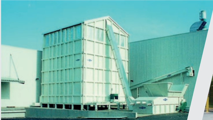
ZENO plant with shredder type ZTLL and infeed hopper. Conveying of wood chips via chain conveyor into a silo with 1000 m 3
