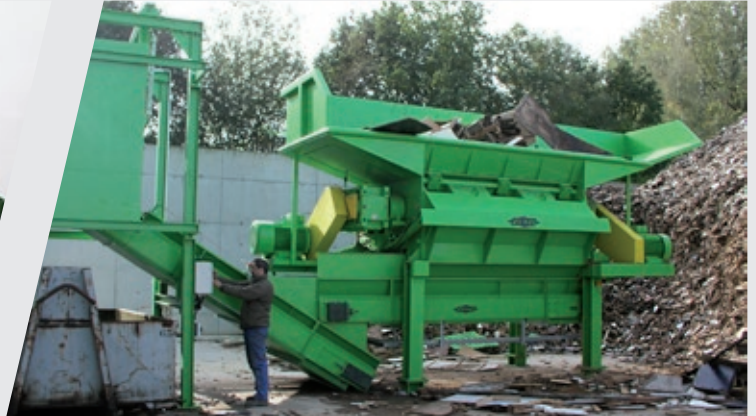
Pre-crusher for waste wood, approx. 50 t/h
