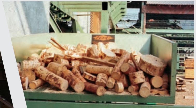
ZENO vibrating dosing feeder with vibratory trough conveyor in a sawmill
