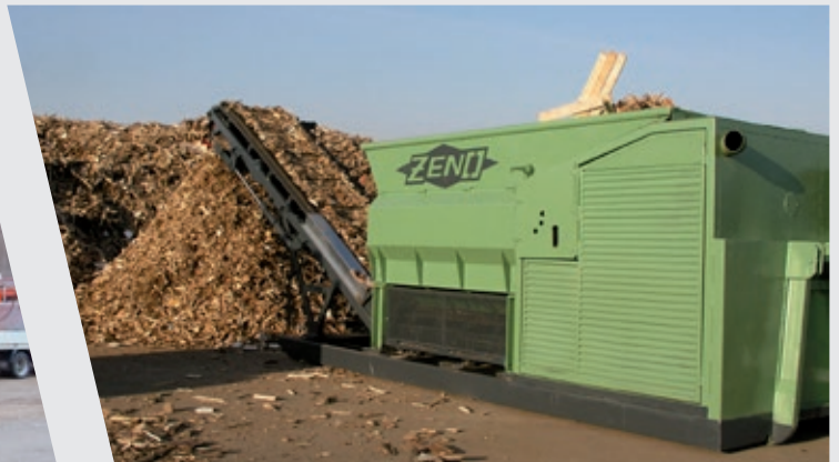
Mobile pre-crusher with Diesel engine
