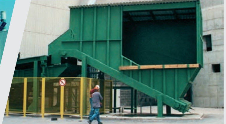
ZENO infeed bunker with screening plant for RDF processing line "wood" in a cement plant
