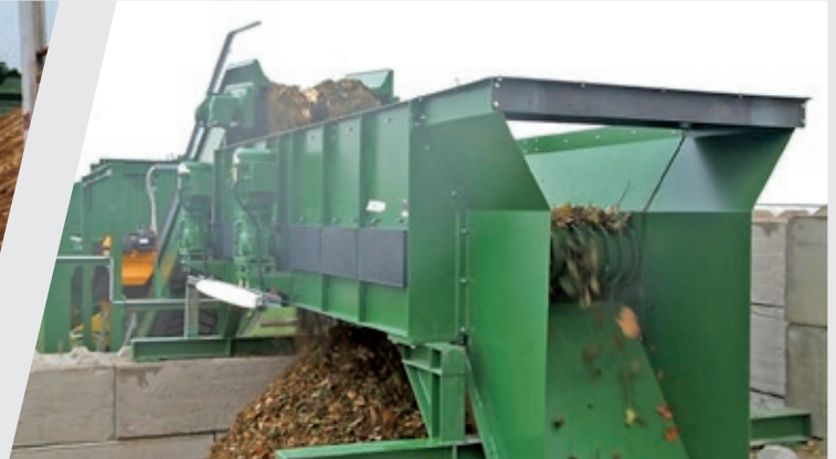
Disc screen for grain size classification of waste and fresh wood
