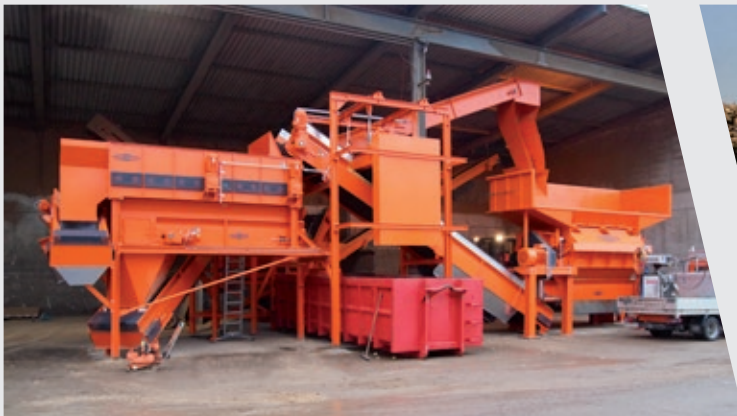
Waste wood treatment plant – in one step to 60 - 80 mm grain size
