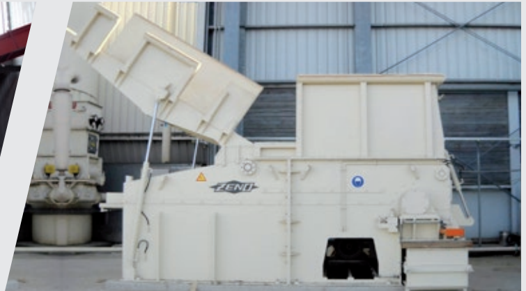
ZTLL for chipboard plants with lifting device
