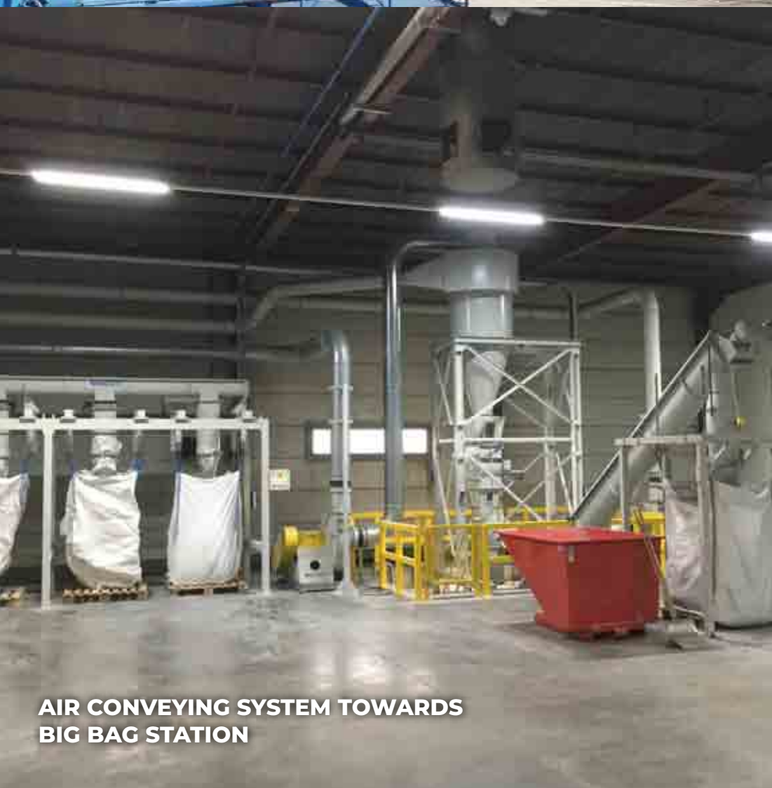
DUST EXTRACTION WITH PNEUMATIC CONVEYING TOWARDS SILOS
