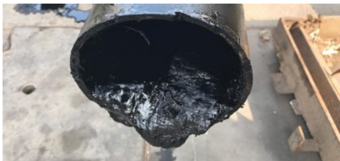
With mineral oil, loose carbon particles gathered in low-lying areas, causing sludge.
