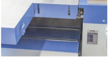
**Option.** The driven table roller can be activated to ensure that short parts as of approx. 320 mm are moved out of the machine.
