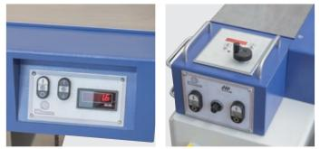
**Simple operation.** Well-structured buttons are used to set the required dimensions for surface (l.) and thickness planing (r.).
