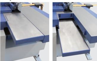
**Quick adjustment.** Segments of the worktable can be adjusted quickly for conversion to the thickness planing function.
