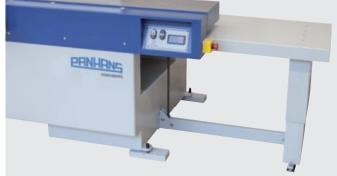
**Option.** The thickness table extension expands the work area by 1000 mm. Height adjustment takes place automatically.
