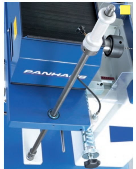
One hand lever operation with remote locking of the dowel boring device for comfortable working
