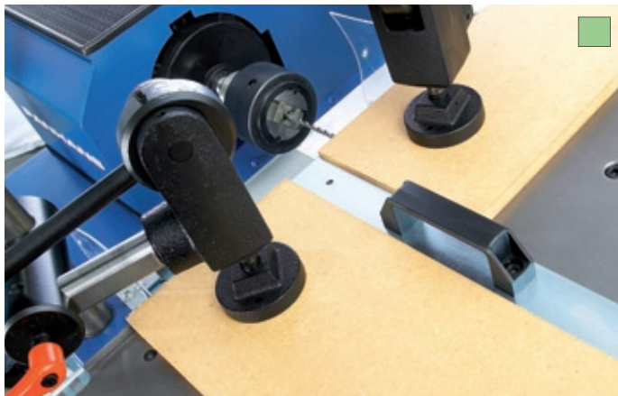
Fence for frames to insert with 2 manual eccentric clamps
