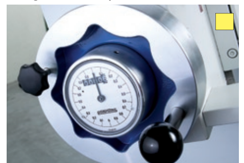
Counter in hand wheel for height adjustment, partition 0.1 mm
