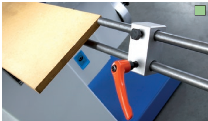
Work piece fence up to 1500 mm long, freely adjustable
