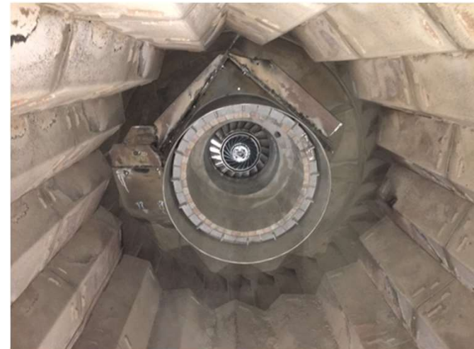
Inside view of the drying drum with the burner
