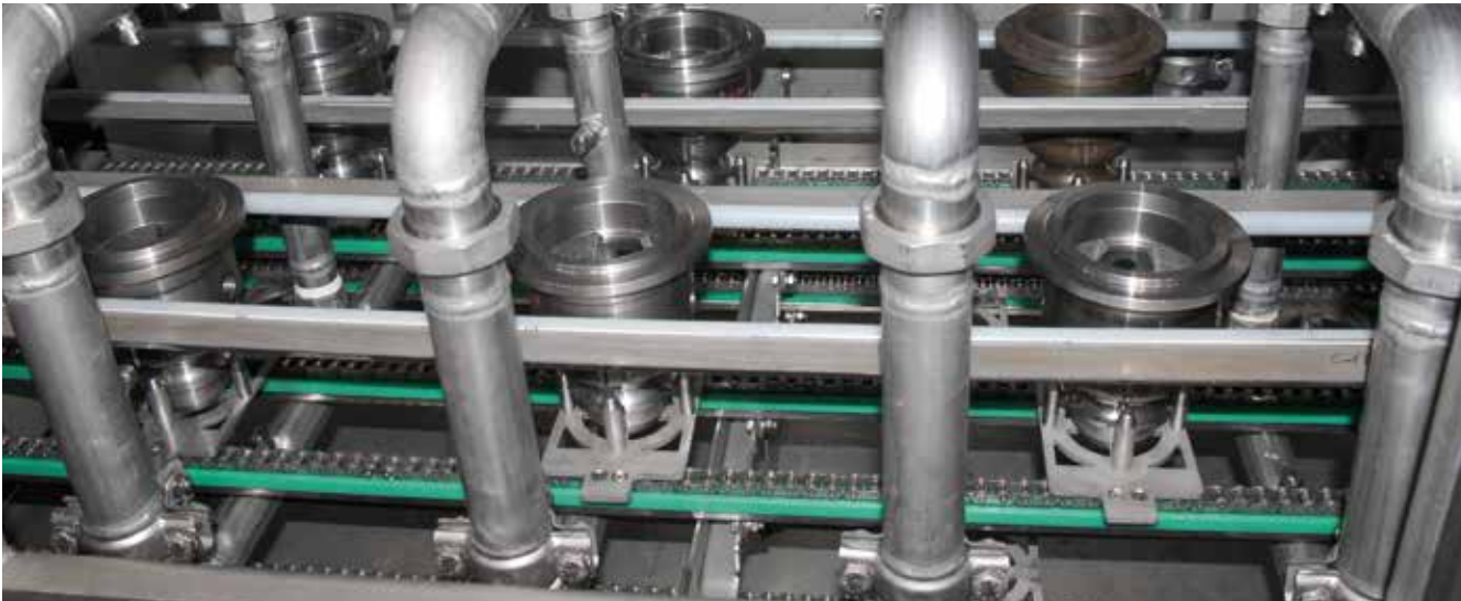
Chain conveyor with bolted-on workpiece carriers and adapted nozzle system
