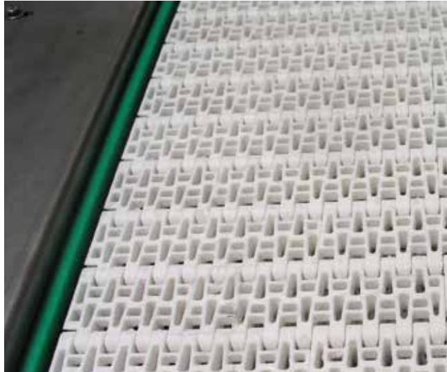
Plastic conveyor for sensitive component surfaces
