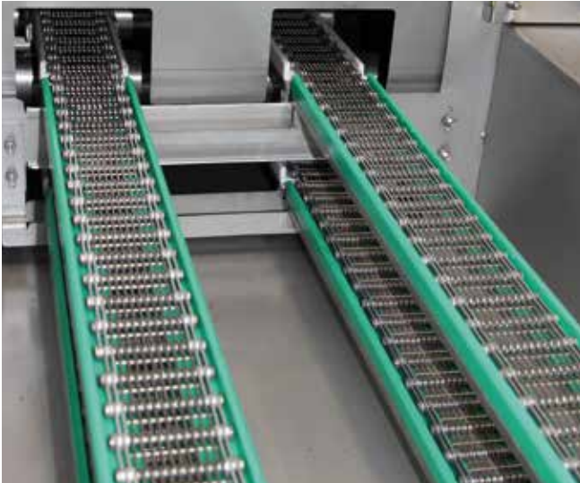
Two-lane mesh conveyor for smaller, different components
