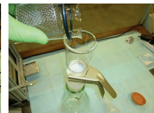
Empty beaker into filtration unit
