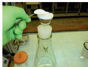
Place filter in filtration unit
