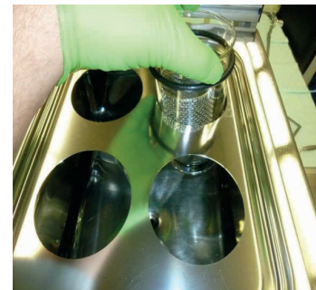
Place beaker in ultrasound bath
