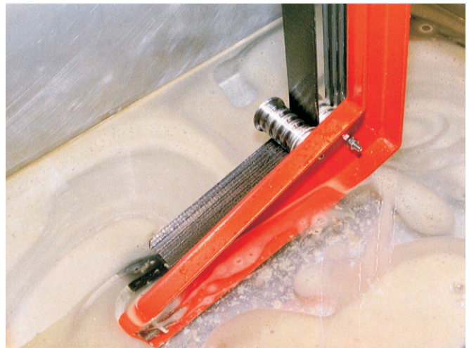
Floating oil sticks to both sides of the belt
