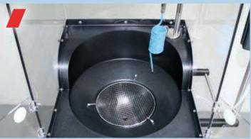
500 mm basin with combinable extraction options such as rinsing, spraying and flooding, incl. a 300 mm ultrasound basin. Optimized surfaces area for low and fast blank values.
