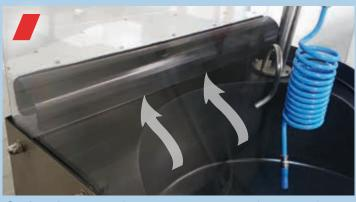
Optional : prepared extraction system at the rear side, increasing operator safety.
