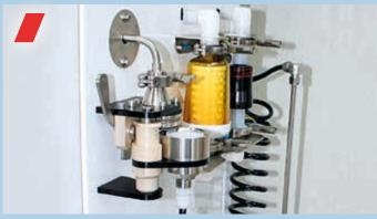
Ergonomic membrane holder can be swung open. Incl. filter cascade for up to 3 analysis membranes. Simple and safe, our procedure for emptying or filling.
