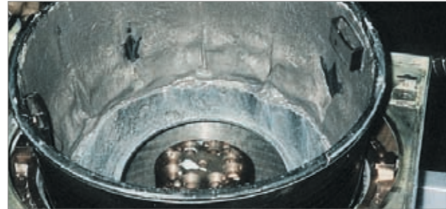
The sludge container of the drum separator can hold up to 5 litres of nearly dry sludge. The container can be changed quickly and is easy to clean thanks to the snap closures.
