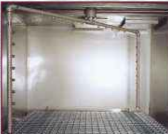
(Standard) Rotating blast pipe system
