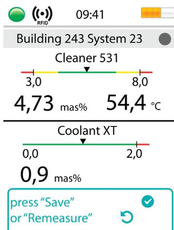
Clear measurement results from a user-friendly system. The current measured value is displayed relative to the specific limit values for the system. The active measurement location is always displayed.
