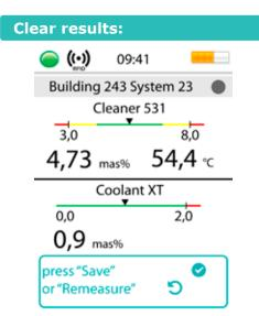
Clear measurement results from a user-friendly system. The current measured value is displayed relative to
