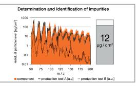
The diagram shows the comparison of signatures of contaminated components with two production supplies "FHM A" and "FHM B". The matching signatures identify FHM A as the contamination cause. The residual amount of dirt is  $12 \,\mu\text{g/cm}^2$ .
