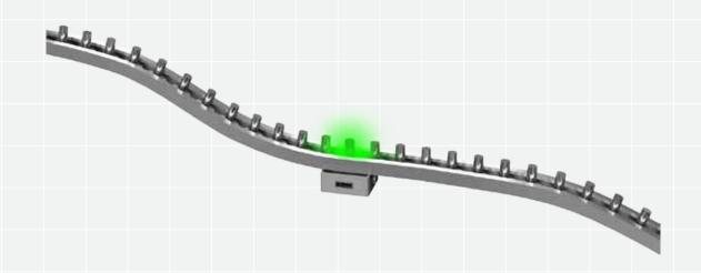
Work pieces are quite often forwarded from one machining centre to another by transport rails. If the work pieces have been magnetized during pre-machining, there will be problems with adhesion, clutching, false orientation, and others during material flow, or at the next stage of production.
