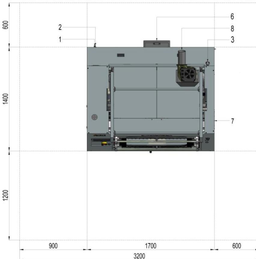
From the front side minimal 1,2 m space for machine operation (and for withdrawal of emergency pan with decanters)
