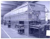
This example of a throughfeed cleaning machine with integrated conveyor technology consists of the the following stations: cleaning, blowing, rinsing, vacuum drying and cooling There are 2 cleaning agent containers under the conveyor belt which have a holding capacity of 2,000 litres each.
