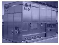
A vapour drier is fitted to the inlet to prevent excessive steam emission at the inlet and outlet. There are servicing hatches on the side of the machine which enable optimum access to the nozzles or the blowers.
