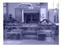
A gravity oil separator is attached to the cleaning container to continuously separate oils and thus increase the operating time of the wash. Large doors are included for servicing and inspection and enable individual components to be accessed easily.
