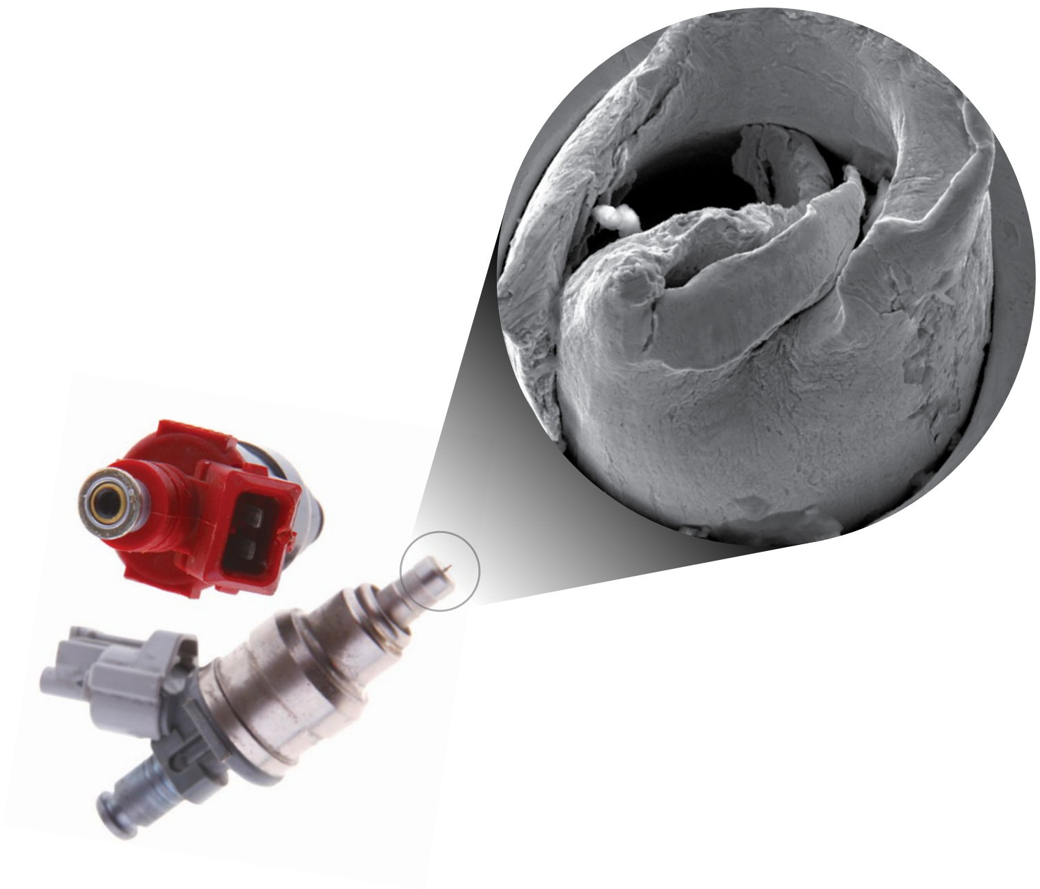
Lodged Particle. SEM image of particle found lodged inside a nozzle resulting in blockage of fuel flow.
