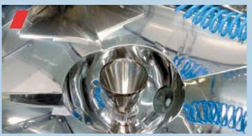
The tank, measuring 700 mm x 600 mm for components up to 15 kg. As on the ACM 17, combinable extraction options such as rinsing, spraying and flooding, incl. a 300 mm ultrasound tank. Optional funnel: small components subject to high demands can be tested more flexibly and quickly
