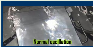
Aluminum foil damaged by Normal oscillation
