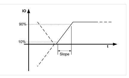
The CRS software produces a controlled Slope in output current to avoid oscillation, overshoot, undershoot or deviation of chosen pattern. In order to simplify choosing, and to introduce a standardization, CRS has divided the Slope time in three values:
