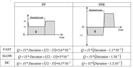
E.g. in a FAST PPR machine that deliver 1ms pulse, the total charge is 11% less than the theoretical expected, in SLOW a 3ms pulse has 33% less charge.
