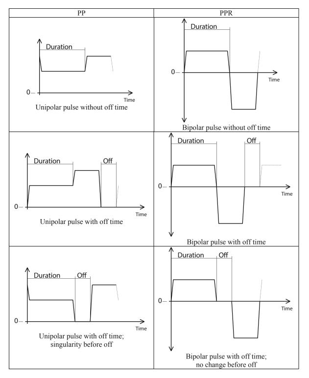
Duration is the time that completes one single pulse or the zero to zero time.
