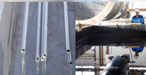
The two locations in Wilhelmsburg and Stellingen are conveniently located and offer cleaning for oxygen applications and phosphating of C-steel constructions. In these processes high quality work is the most important requirement. Because of extensive inspection methods, organic compounds on the surface are determined and thus the predefined specifications can be observed.
