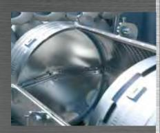
The surface quality of stainless steel equipment is very important because of direct contact with the product. Electropolishing significantly improves integral properties of your equipment. Very shiny, almost inert stainless steel surfaces arise from the electrochemical process. Electropolished surfaces are also very suitable for decorative purposes.
