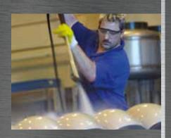
**Pickling** is used to remove all impurities from stainless steel surfaces with the objective of obtaining a pure metal surface. A protective passive layer can only be formed on such pure metal surfaces.
