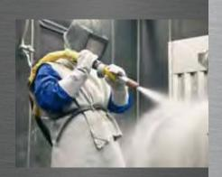
Glass blasting is a mechanical surface treatment that is particularly well suited for achieving an equal and even look. Welding spray, rust, scale and annealing colours are easily removed. With this treatment the surface is not only cleaned but also solidified so that the resistance against tension crack corrosion is increased. The smooth and hygienic surface properties resulting from this treatment are interesting for the food and chemical industries in particular.
