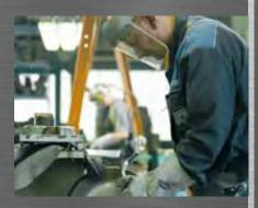
By grinding stainless steel, we obtain visually and functionally good quality surfaces with a defined roughness as required in some industries, particularly the pharmaceutical industry. Treatment to give surfaces a mirror finish for decorative purposes is also available.
