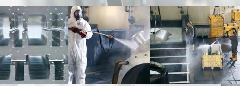
We specialise in on-site pickling and cleaning of pipes and vessels, particularly in the fields of pharmaceutical or food processing companies. Cleaning, electropolishing and pickling, can also be done on-site and are carried out environmentally sustainable.
