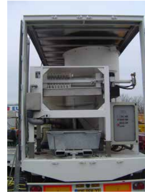
Filtro pressa montato sul camion Filter press on a truck for purifying
