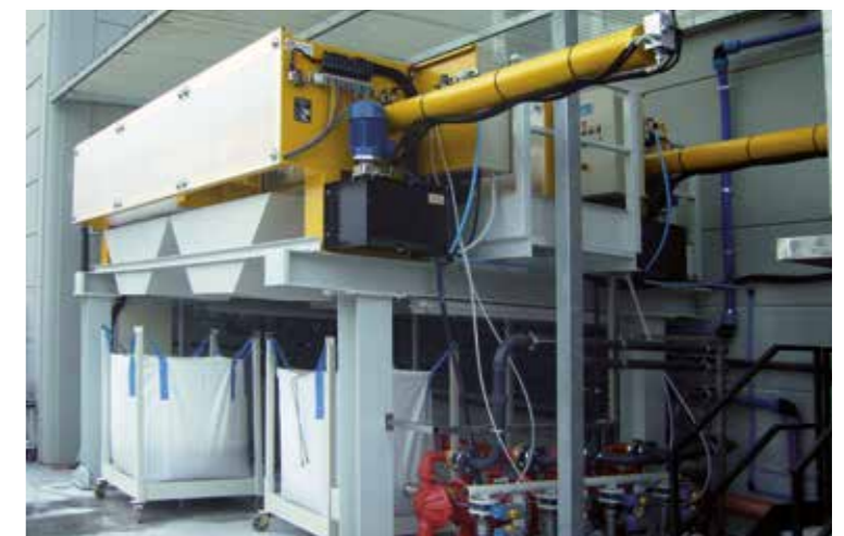
Filtro pressa con scarico in big-bag Filter presses with discharge in big- bag
