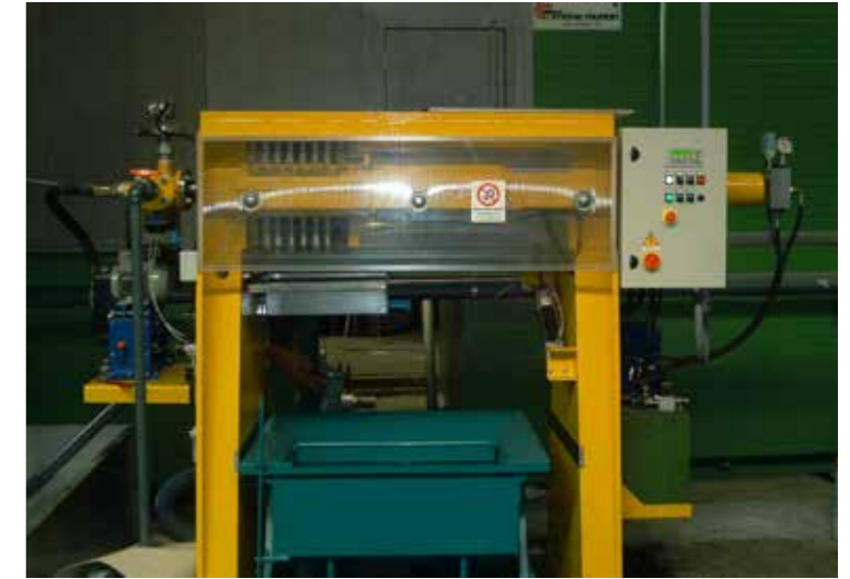
Filtro pressa con scarico in contenitore Filter press with discharge into wheelie
