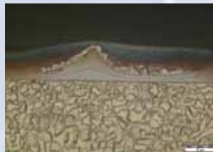
Ground sample of a nickel-plated brass component: substrate inclusion in the coating
