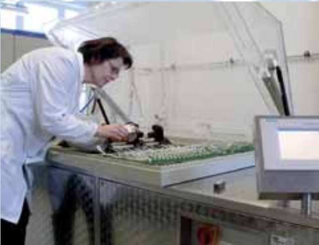
Interim assessment during a corrosion test
