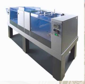
The laboratory bench systems of series MINISTAR and the floor-mounted units of the series ETCHING CENTER V are used for developing, etching and rinsing in foametching process and continuous development process. They are ideal for the processing of small printed circuit boards and etched plates in laboratories, schools and institutions to create professional sample sheets and prototypes.
