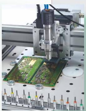
Lemmen's compact brushing machines can be used universally for different materials and substrates include laminating or deburring, after drilling in the print production. Special devices of single or double-sided working table units or floor units are also available.
