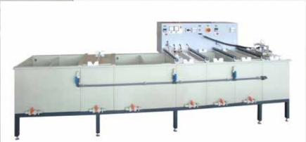
a pre treatment tank for degreasing and rinsing cascades. Optional items like exhaust tubes and suction heads provide a clean work environment.
